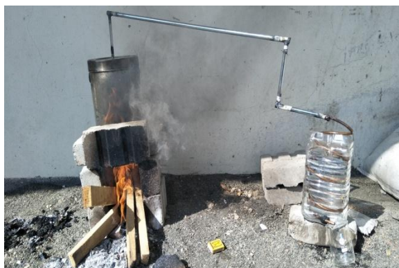
Fig.5. Homemade setup of Pyrolysis process.
